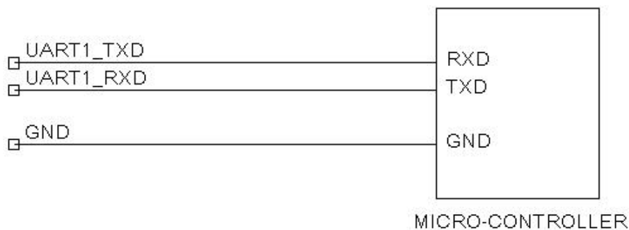
Figure 5-1 UART interface and microprocessor connection reference design
